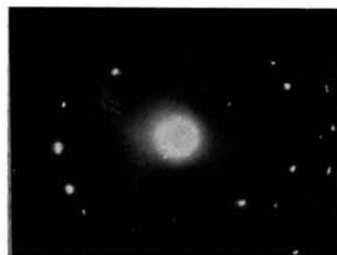
Fig. 18(b). Diffraction pattern from a BeO flake.
