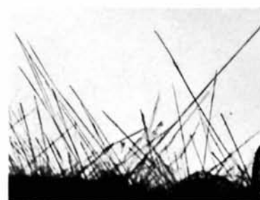
Fig. 16(a) Electron micrograph ( \times 14,000 ) of Be crystal heated at 800 °C. for 1 hour, showing needle-like growth.
