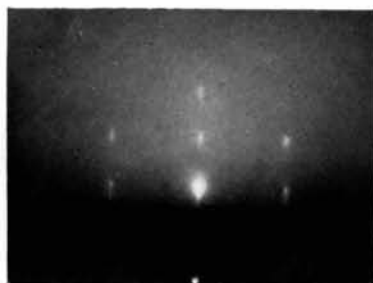
Fig. 1. Be(001) cleavage face; beam along \langle 100 \rangle .
