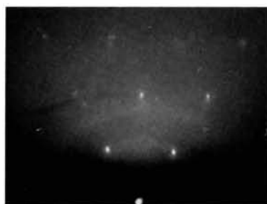
Fig. 14. Electropolished (110) face; beam along \langle 001 \rangle .
