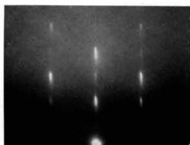
Fig. 9. First electropolished (001) face; beam along \langle 100 \rangle .
