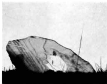
Fig. 18(a). Electron micrograph ( \times 5,000 ) of BeO flake.
