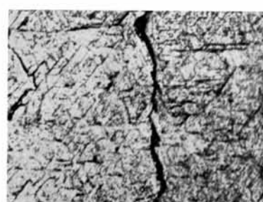
Fig. 7. Be(001) cleavage face, after heating at 800 °C. for 30 min. ( \times 130 ).
